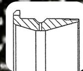
Flanged double cup to accept two taper roller cones, with oil groove and oil holes.
