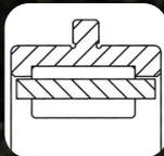
Roller bearing with flange in middle of outer race diameter, with locating slot and one piece bronze cage.
